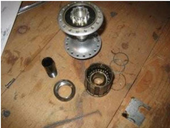
Here's the hub with the hollow bolt, and the bearing cup removed.
