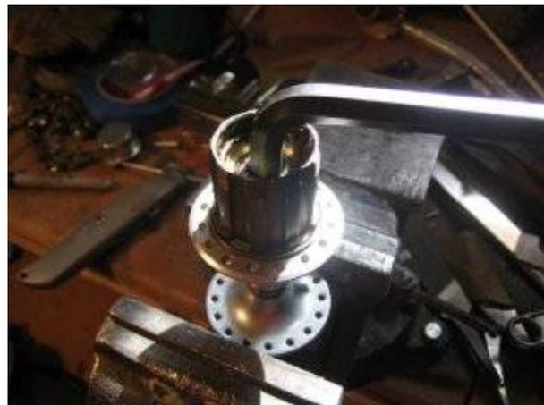
The freehub needs to be taken completely apart so the palls can be removed. This allows will allow the freewheel to spin in either direction.
