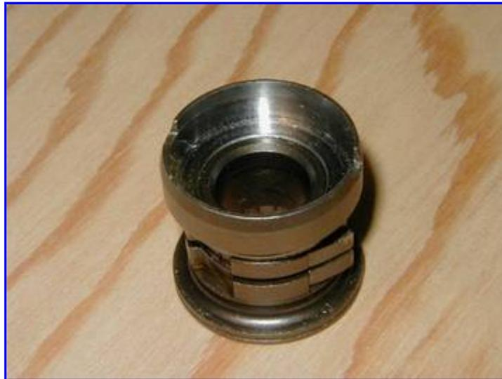
A sealed bearing can be used. Heat the main bearing to remove the hardness, and then machine to ~1.02" inner diameter. A sealed bearing would slightly reduce the width of the freewheel.
