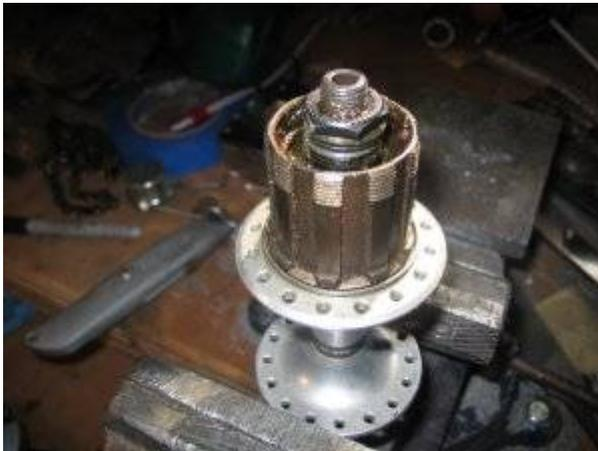
First remove the gear cluster assembly. You may need the special Shimano cluster tool to accomplish this, as well as a chain whip tool.
