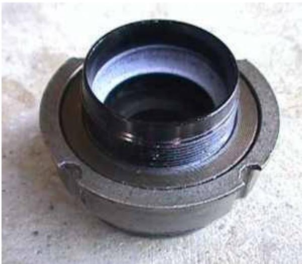
After you screwed the bottom bracket retainer into the freewheel, you can just screw that into a bottom bracket.
