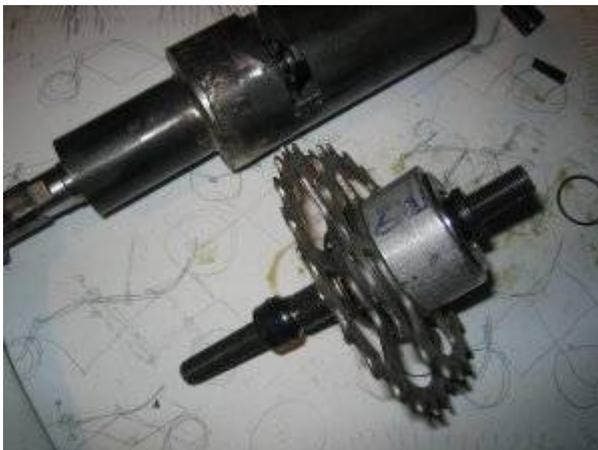
Here is the completed intermediary jackshaft. I used a couple of spacers between the two gears to ensure they were far enough apart that the chains would not rub. I made a big lightweight spacer for the remaining space on the hub with some handy aluminum tubing.
