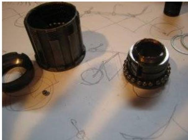
Cut the threaded section off of the hollow bolt. It will be used as a spacer. You will need to use a cut off
