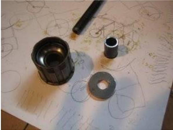
tool or dremel rather than a hacksaw, as the hollow nut is made of hardened steel. Make a thick washer, which will go on the bottom of the freehub.
