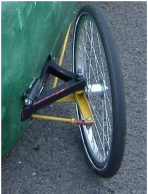
Bear in mind this is very crude, and allows for no castor or camber adjustment.
